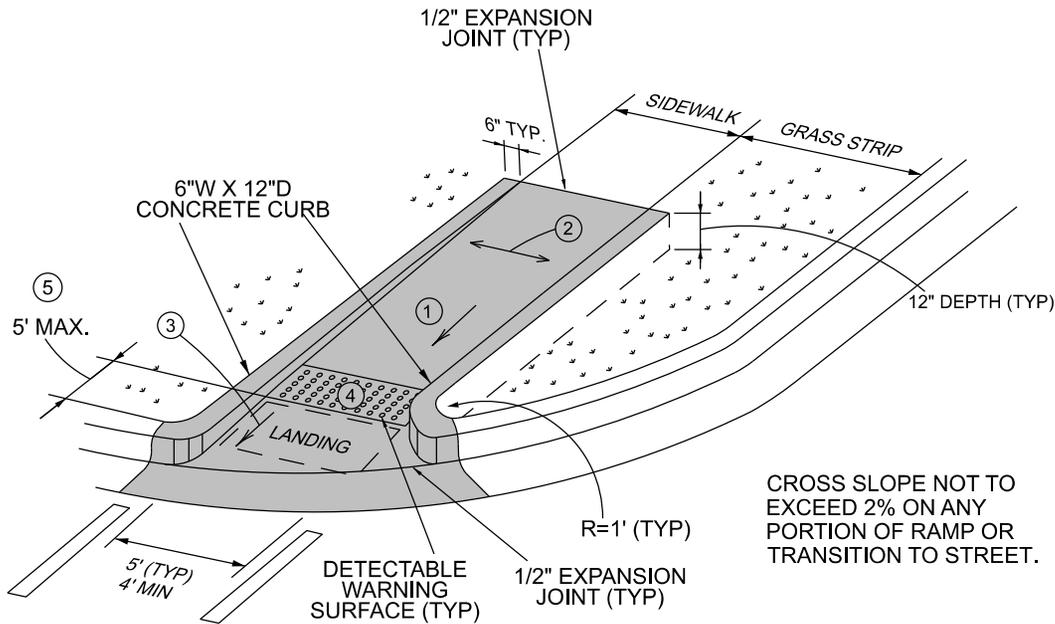
CROSS SLOPE NOT TO EXCEED 2% ON ANY PORTION OF RAMP OR TRANSITION TO STREET.
