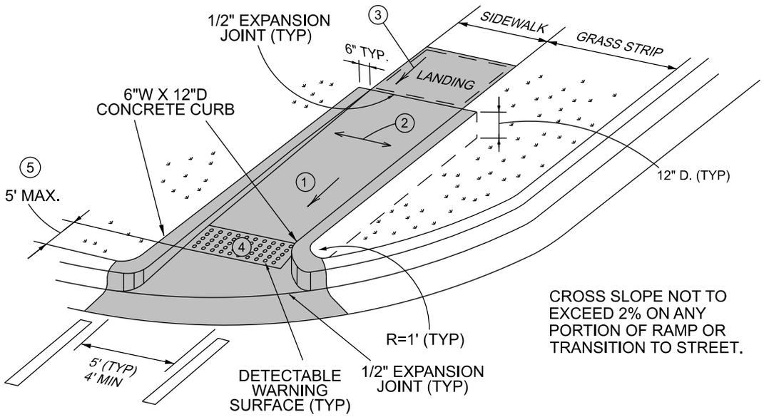
CROSS SLOPE NOT TO EXCEED 2% ON ANY PORTION OF RAMP OR TRANSITION TO STREET.
