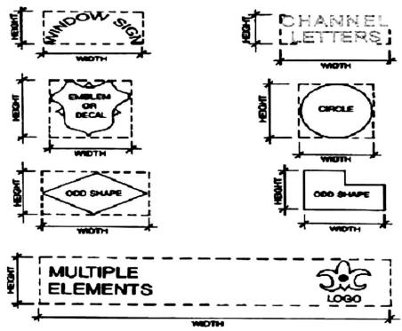
**Signs attached to walls.** Where a sign consists of individual letters, words or symbols attached to a surface, building, canopy, awning, wall or window, the sign area shall be the area of the smallest rectangle which completely encompasses all such letters, words or symbols and any accompanying background of a color different than the natural color of the wall.
