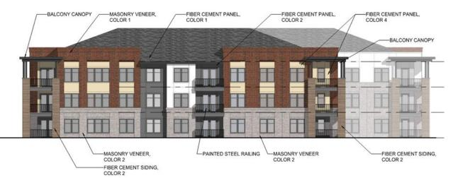
Elevations provided for each building façade and each building along with material calculations in keeping with architectural zoning conditions
