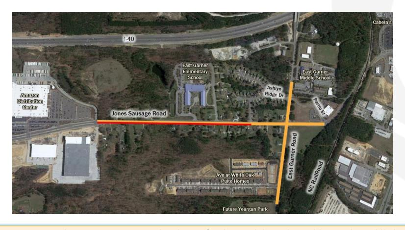
Jones Sausage Road Improvements – road widening for the north bound travel lane only, middle lane remains for turning. 5-foot sidewalk, curb and gutter will be added along the east side
