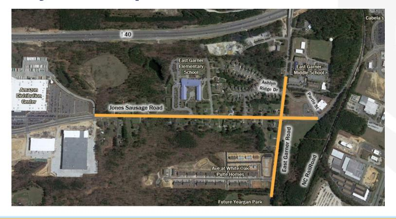
**Jones Sausage Road Improvements** - widened to a four-lane, median divided facility with a 5-foot sidewalk on the east side, and a 10-foot multi-use path (MUP) on the west side from Amazon to Partlo St
